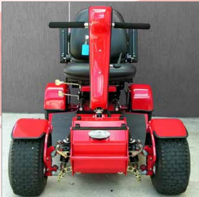
70mm of travel in the front suspension.
