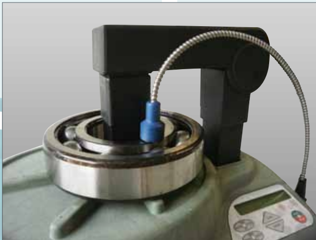
Measuring bearing temperature via temperature gauge.
