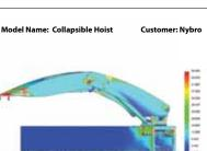
tudy Name: Lifting Capacity lot Type: Static Nodal Stress One lobal Value: 0 to 1132.96 N/mm^2 (MPA)
